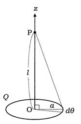
(1) Find the electric field produced by the charge on small arc  $a d\theta$  of the circumference at point P located on z-axis with distance l from origin O.
